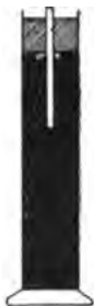
FIG. 54.— Arrangement by which the transformation of the properties of mercury is obtained by combination, under the influence of slight pressure, with traces of magnesium.
